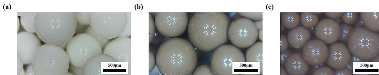
Fig. 4. Optical images of (a) P(St-co-DVB), (b) HCP-TMOF and (c) HCP-DFDA.
