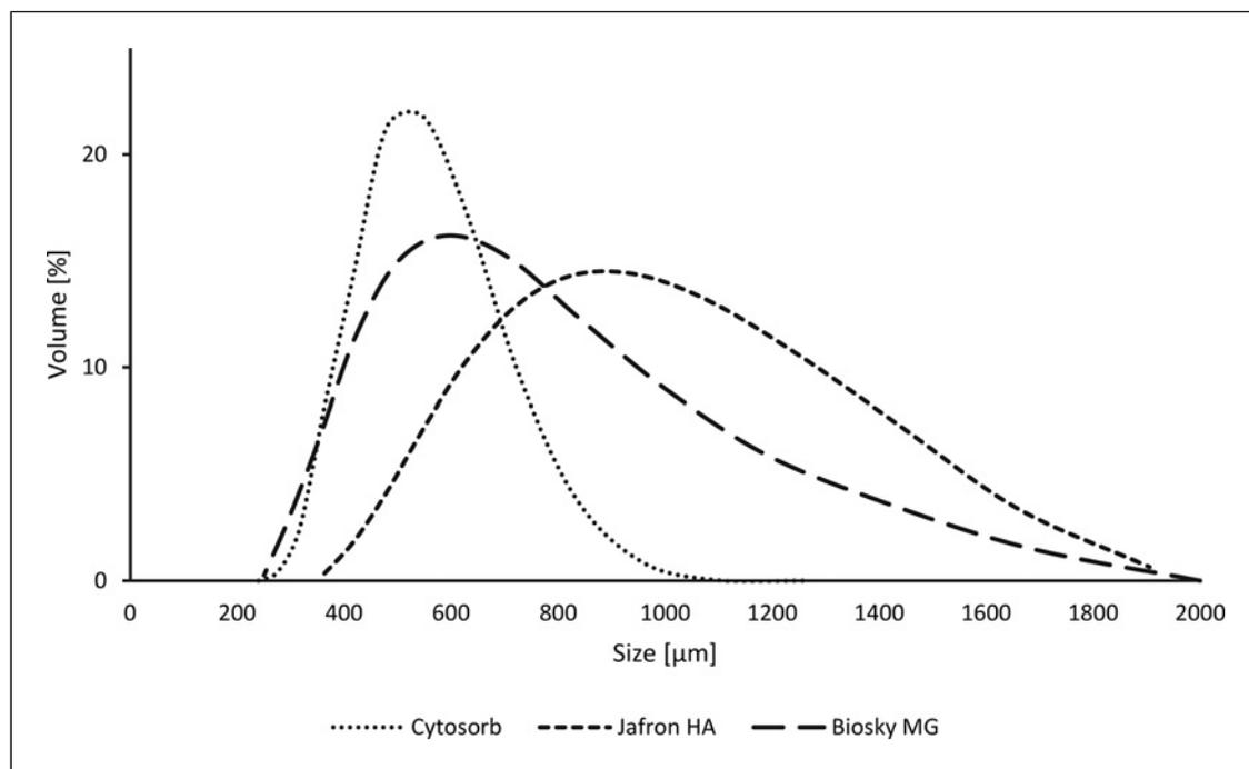
**Fig. 1.** Volume-size distribution of the hemoperfusion adsorbents Cytosorb, Jafron HA, and Biosky MG.
